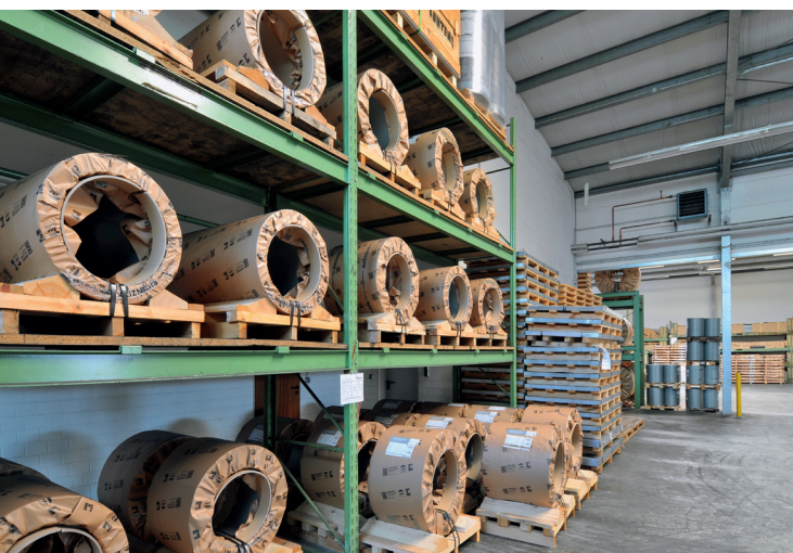
Storage of coils with wooden sleepers
